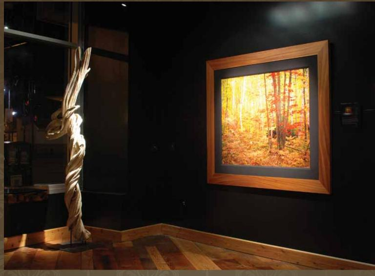
WAC MR16 track luminaires were used with Ushio MR-16 Eurostar™ IR Series of halogen lamps to provide the lighting intensity needed and to comply with California's Title 24 energy efficiency code.
