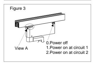
3. To secure the fixture to the track turn the lock switch to its locked position. (See View A)
