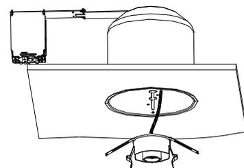
Wing springs hold and center the socket cup inside the housing.
