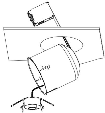
Use fingers then screwdriver to push housing clips to extended position
