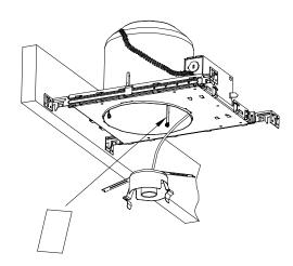
After mounting the housing, use metallic adhesive tapes to seal the slots in the canisters. (Shown above)
