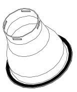
Use the adhesive foam strips to form a ring around the rim of the trim ring. Strip should be on the side making contact with the ceiling surface. (Shown above).
